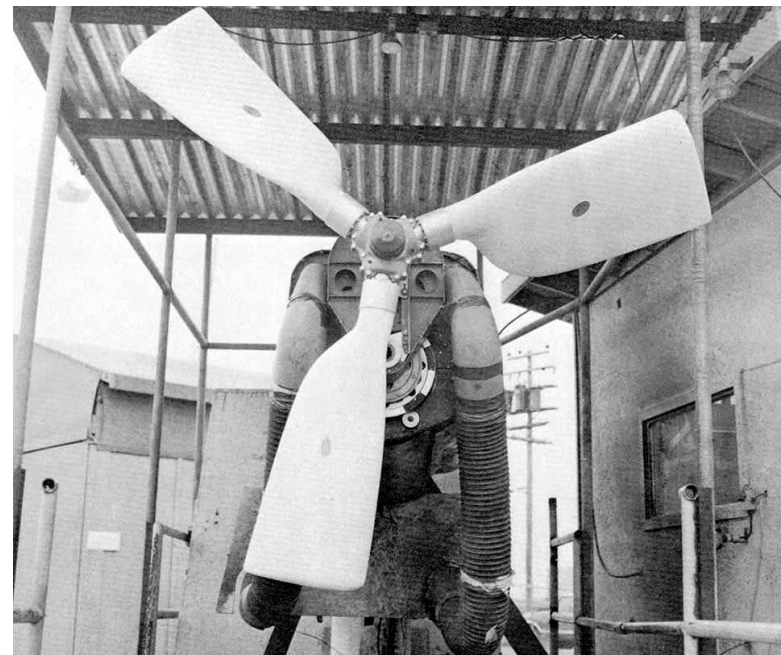
Right: Special acoustic propeller on YO-3A Engine in Test Stand: 100 In. Dia, 13" Chord.
